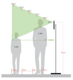
Recommended Installation Height: 150cm Temperature Measurement Distance: 30cm to 120cm
