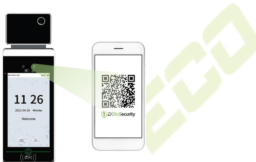
**NOTE:** Place your phone within 15-50cm of the device (distance depends on the size of the phone screen and the density of the QR code). Do not block the camera and the QR code.
