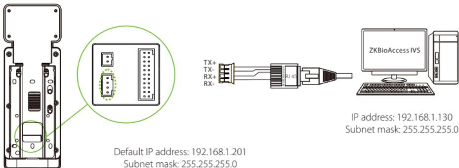
Click [COMM.] > [Ethernet] > [IP Address] , input the IP address and click [OK].
